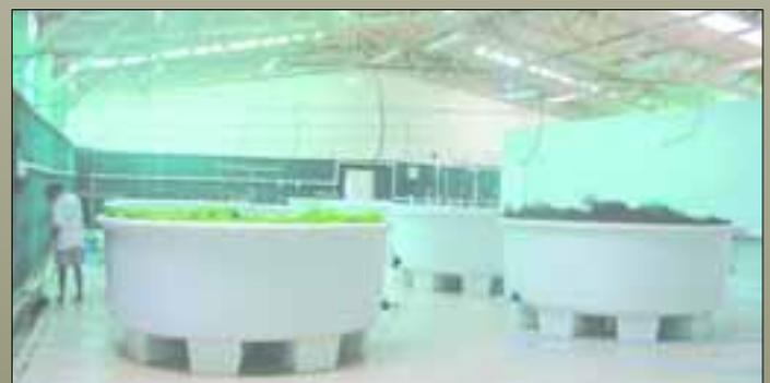
*Internal view of the hatchery at Samarai. Notice the large tanks for rearing the oyster spat and larvae. All these were prefabricated and brought in from Australia given the limited time and the specialized nature of some of the equipment.*
